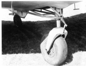
Above: A member of the Horten ground crew tries out a pressure suit developed by the brothers, which was never used in flight. Left: Cockpit interior of the Ho 9 V1. From left to right are fine and course altimeter, turn and bank indicator, vertical speed indicator and airspeed indicator. A compass is mounted below the center. Below: Close-up of the nose gear without covers. Just visible, next to the venturi tube, is the panel which was to be transparent allowing the pilot to visually check the runway distance while landing.
